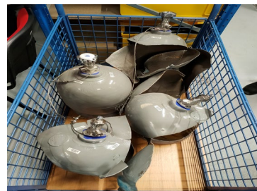
LP cylinders after the accident
