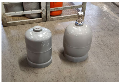
Normal (left) and deformed LP cylinders after leak test (right)
