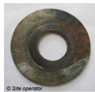
© Site operator Flange's seal upline of the flow meter
