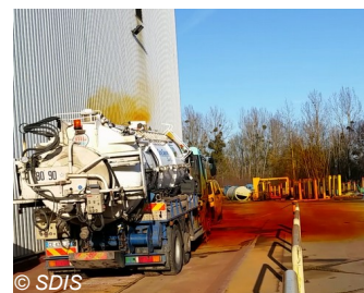
© SDIS Release of nitrous vapours following an unsupervised unloading operation (ARIA 49018)
