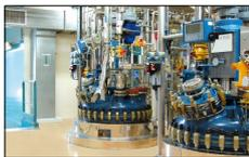
During the manufacturing of an organomagnesium compound, a substance used by the pharmaceutical industry, a non-conforming mixture was formed in a reactor. It was cooled in order to control the reaction, but the reaction intensified after several days, causing the reactor's rupture disc to explode. The series of technical and organisational errors that led to this incident caused the operator to look closely into these highly sensitive exothermic reactions.
