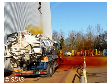
© SDIS Release of nitrous vapours following an unsupervised unloading operation (ARIA 49018)
