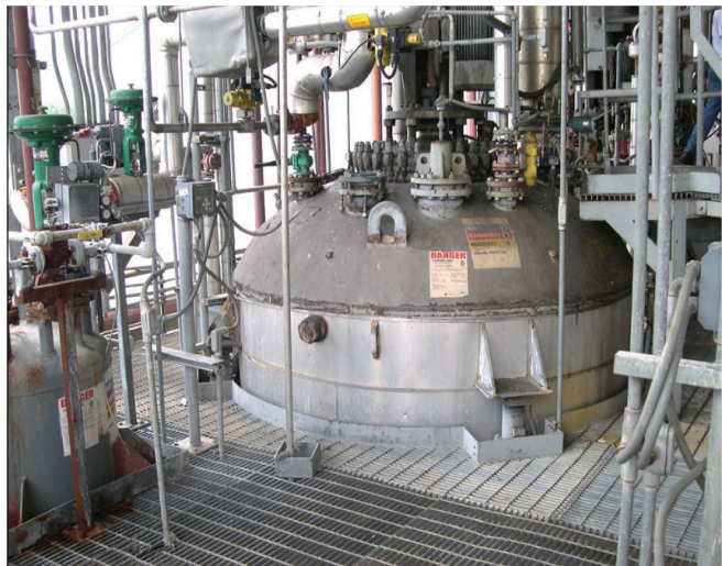
Reactor inside a modern French chemical facility: its loading and monitoring are remotely supervised from a control room
