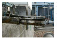
Fig. 4: The fouling of vibrating fork level probes caused a runaway reaction (ARIA 19339, Source: DREAL)
