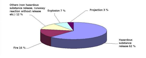
Fig. 2 : Breakdown of phenomena caused by accidents involving sensors (ARIA base)
