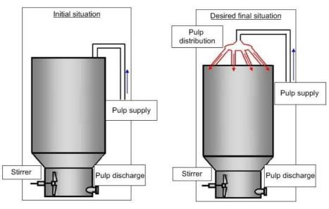
At 8:20 am, in preparation of this works, technicians turned off pulp supply into the tower and proceeded with a 10minute sequence of pipe rinsing with water. This procedure consisted of rinsing all process equipment by injecting 20 to 40 m<sup>3</sup> of water into the pipes, thus adding to the quantity of pulp already present in the tower.
