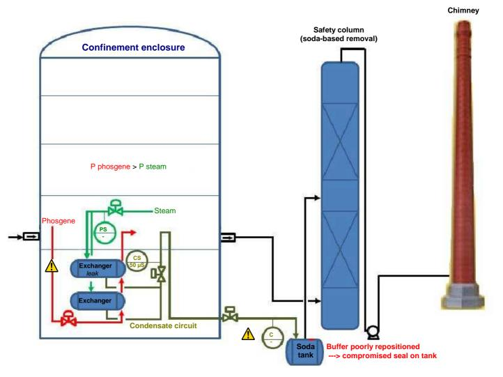
Sensor measuring condensate conductivity with a safety action programmed at 50  $\mu S \to \,$  isolation of the condensate circuit and shutdown of the phosgene pump
