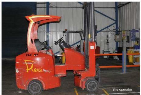
Figure 2: Unprotected electric flexi-truck in use at the site
