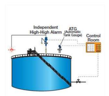
Figure 7: The American API 2350 Standard classes as Category III any storage tanks managed remotely; moreover, it recommends use of a high-high level safety sensor that is independent of the operating level (ATG) sensor and, preferably, offers self-diagnostic capacities relative to its malfunctions and defects.
