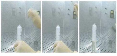
d) e) f) Fig. 10: Gas overpressure after anaerobic fermentation in sealed BES samples ampoules (source: ARPA Puglia)
