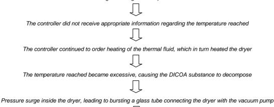
Release of a portion of dryer contents inside building B45, and then to the outside
