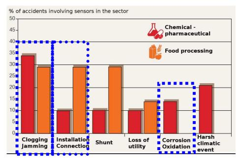
Fig. 5 : Primary causes of sensor malfunction for the chemical and food processing sector (ARIA base)
