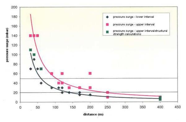
Estimation of the effects of overpressure by INERIS from damage during the Dagneux accident.
