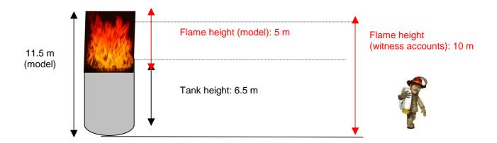
In assuming that the fire duration (10 minutes) exceeded the 2-minute threshold that defines the boundary between the thermal dose approach and the heat flux method (see diagram below), the following results are obtained for the generated heat fluxes.
