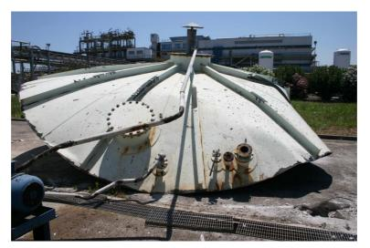
Fig. 9: Exploded roof, note the absence of plain flange on the air line (source: ARPA Puglia)
