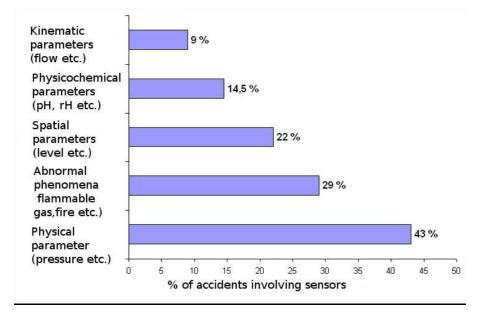
Fig. 3 : Breakdown of the functions performed by sensors involved in the analysed sample of accidents (ARIA base)
