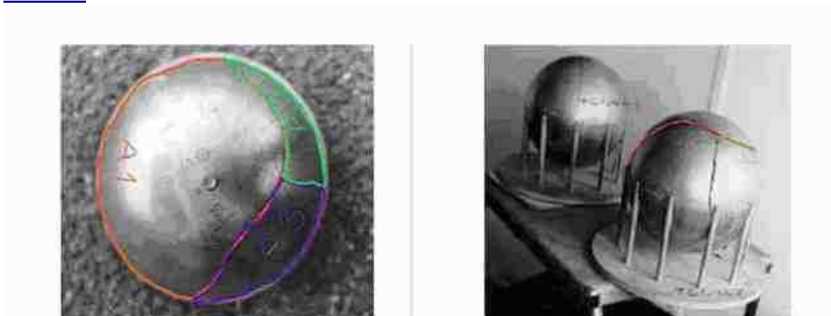
Figure 19 – Model of the main fragments of sphere T 61442
