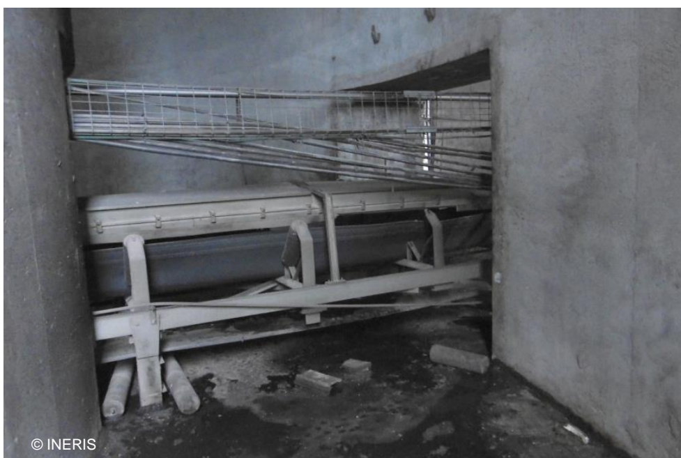
Traces of combustion in the sub-cell gallery
