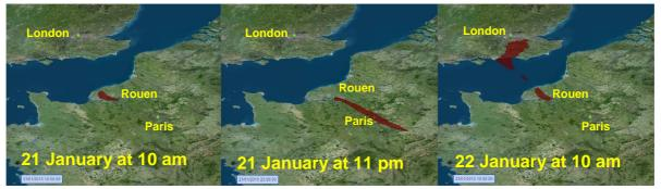
Fig. 9: Modelling of the foul-smelling plume (shown in red) between 21<sup>st</sup> and 22<sup>nd</sup> January (Ineris)
