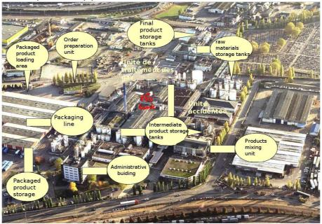
Fig. 2: Main plant installations (site operator)
