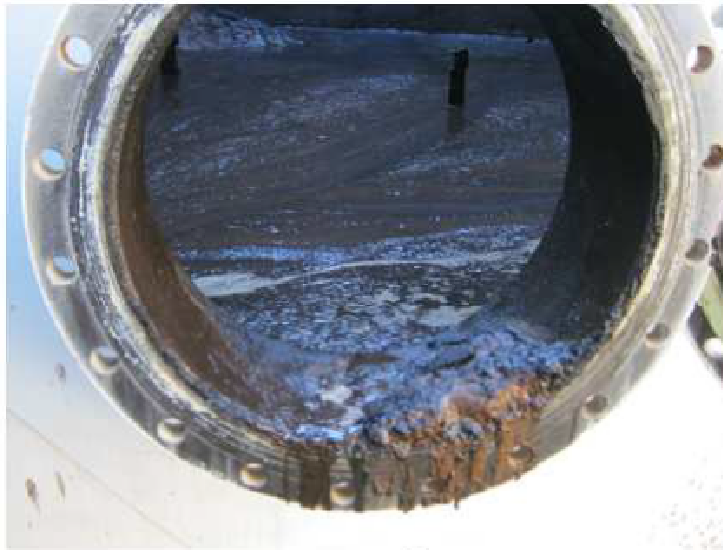
Fig. 12: Solid / paste residues collected from the exit nozzle (source: operator)
