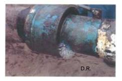
The investigation, as carried out by the Inspectorate of the Ministry for the Environment, has provided evidence that an underground pipeline, in which hydrogen gas is transported, developed a leak resulting in an escape of hydrogen gas. The leakage lasted for at least several hours but it can not be excluded that the leakage started weeks or even months prior to the discovery of the leak.
