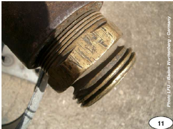
Examples of worn bolted connections : connector at tank end and bolting ring.
