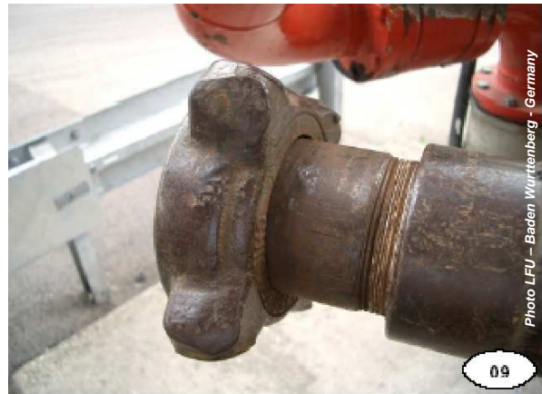
Examples of worn bolted connections : connector at tank end and bolting ring.
