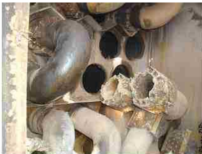
View of a peripheral elbow on the convection chamber (after the fire)
