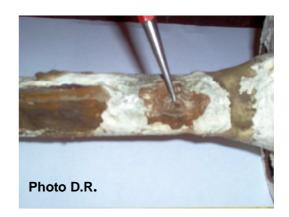
No structural or chemical composition anomaly can explain the type of corrosion. The hypothesis by default in this case is that of a rainwater retention point owing to the geometric configuration. A stagnant drop on the "ceiling" triggers a differential aeration mechanism, known as the "Evans drop", resulting in local acidification. This leads to "blistering" of the paint at this point and localised cavernous corrosion of the substrate.
