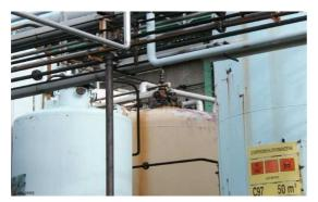
Having noted that the transfer pump was malfunctioning, the GLCF technician stopped the operation and began spraying down the tank with the sprinkler system. The personnel noted a small explosion, probably due to excess pressure in the tank, and a cloud of acid gas was released through the faulty flange seal on the upper dome of the tank.
