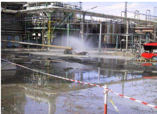
Dilution of NH 3 by water curtains
