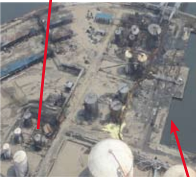
The fire spread to the petrol, liquid sulphur and bitumen storage tanks. A tank tilted to one side by the tsunami collapsed while burning (Source : NRFID)
