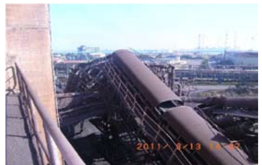
Damage to the sinter conveyor (Source : Sumitomo)
