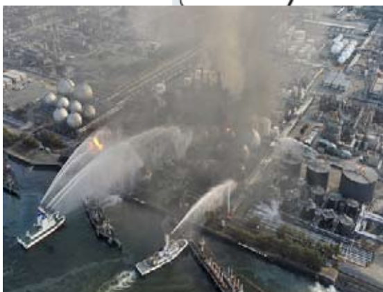
Fireboats extinguishing the LPG tank farm blaze. The wind coming from the sea made extinguishing the fire from land impossible (amateur photo)
