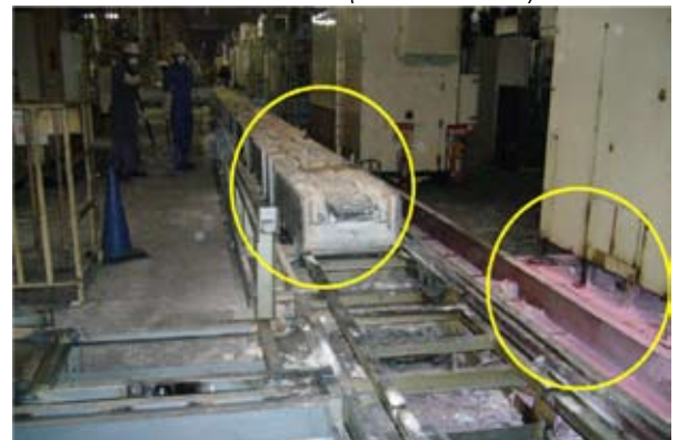
Drop of overhead carrier (Source : Nissan)
