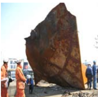
View of a BLEVE from the opposite side of Tokyo Bay (estimated diameter of the largest BLEVE: 600 m). Below: piece of a sphere. (Source : NRFID)
