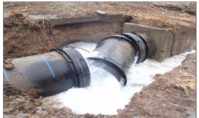
A 2400 mm (96") drinking water pipe that burst despite being fitted with a 500 mm deformable flange (Source : Miyagi Prefecture)
