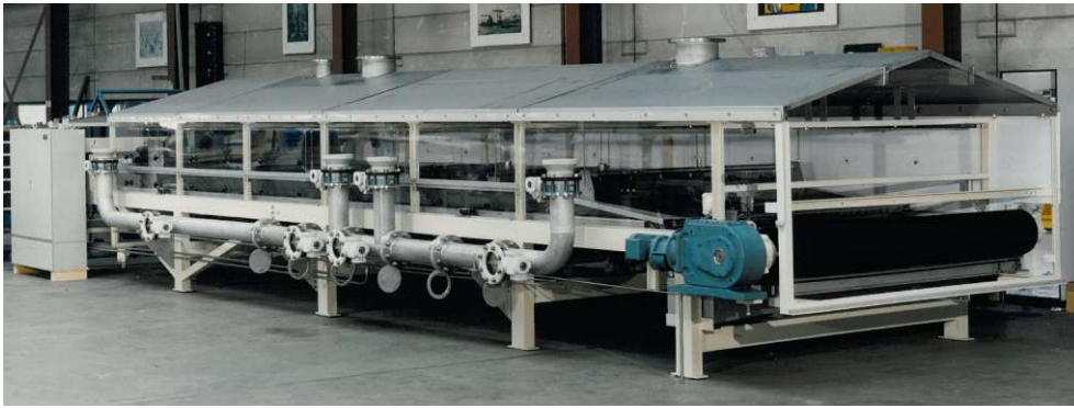
Generic illustration of a RT vacuum belt filter (Picture Larox Pannevis R.R.)
